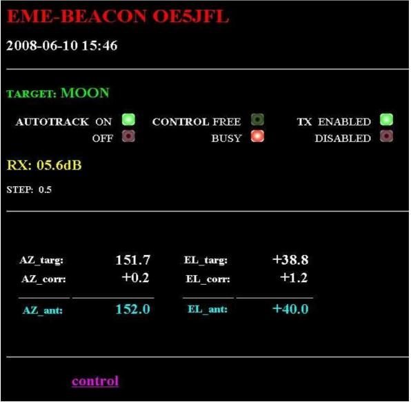
This page is refreshed every 5 seconds automatically, it shows you the position of the moon (or the sun), the position of the antenna and it's correction values, and some status lamps.
